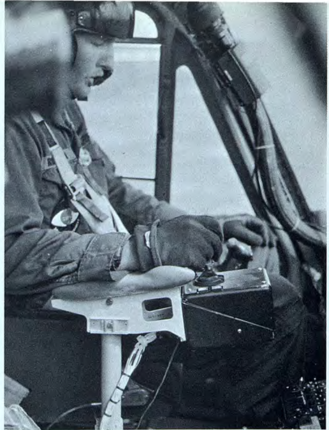
An Infant pilot adjusts the infrared search light while monitoring the television receiver.
