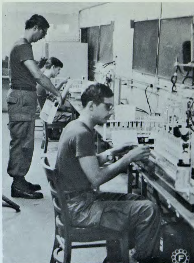
Technicians at the 9th Medical Laboratory perform various phases of the Thin Layer Chromatography (TLC) test. When sprayed, morphine will appear as a blue stain on the plate.
