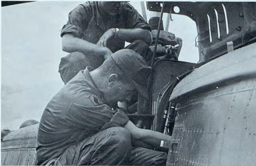
SFC Norman Lister inspects the hydraulic system on a UH-1H Huey.
