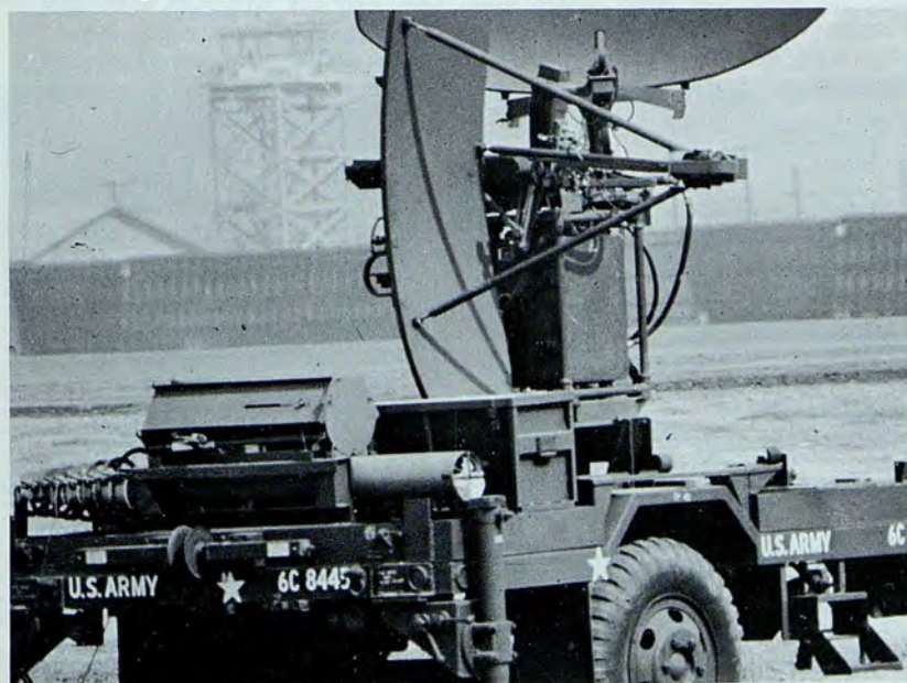
Ground Control Approach radar picks up aircraft and transmits an image to the GCA Specialist's radar scope.
