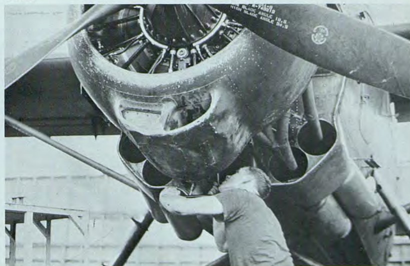
A crew chief works on the exhaust system of a U-1A Otter of the 54th UAC.
