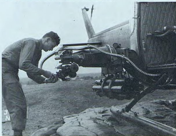
The XM-21 weapons subsystem consisting of 7.62 minigun and 2.75 inch rocket pods.
