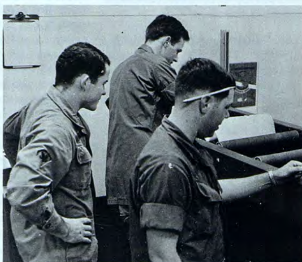
The editor-operators use a "decolator" to separate the computer's data output.
