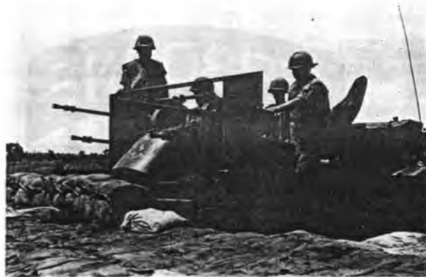
The Quad .50 caliber machinegun mount is capable of unleashing more than 2,000 rounds per minute.
