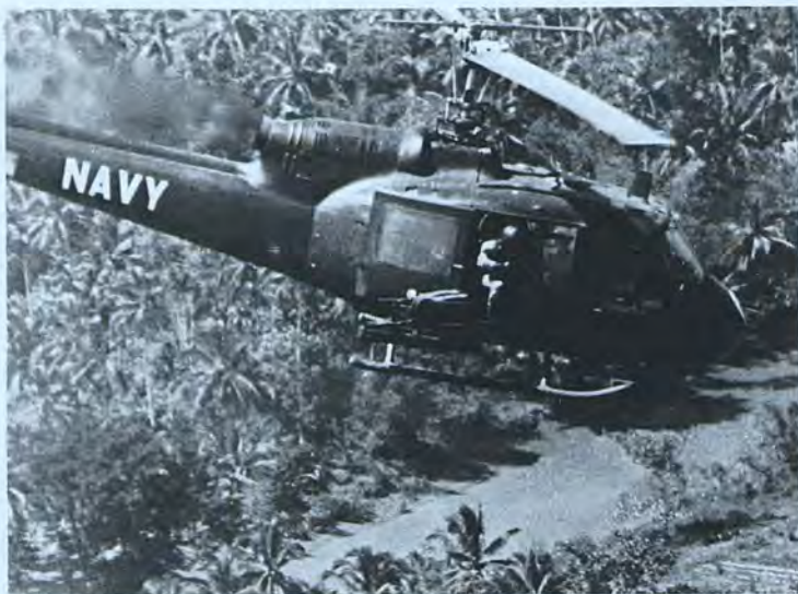
Seawolf helicopter gunship sweeps low over Vietnam's Mekong Delta with its door gunners ready. HA(L)-3 operated a total of nine gunship detachments during the Vietnamese conflict. This helicopter is equipped with the M-16 armament system. (Via Bell Helicopter)
