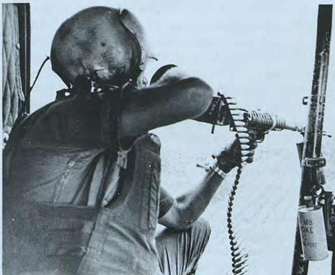
Det 4 door gunner fires on a target, November 1967. Note how this hand-held M-60 has been modified to fire sideways. This caused the shell casings to be ejected downward, away from the helicopter's main and tail rotors. (U.S. Navy)
