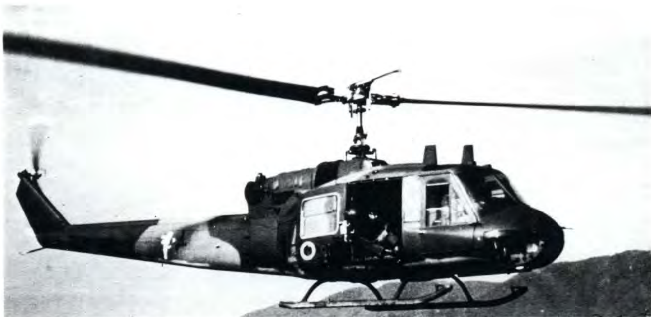
This Bell UH-1P (65-7935) has a universal mount for its cabin gun but without the dust shield on the outer face. The Sagami mount is hinge-fitted to the forward end of the universal mount. The boom marking includes a Mexican character "swatting" the hornet. (Photo via Bob Chenoweth.)
