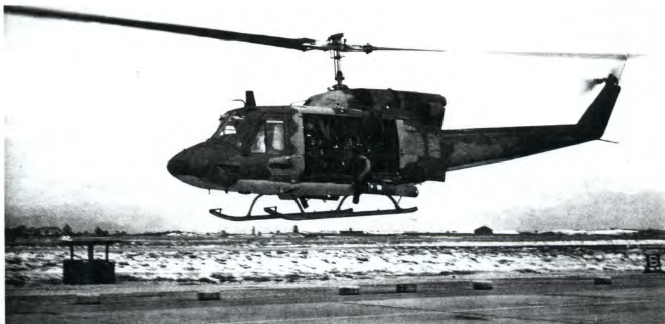
A UH-1N operating at Cam Ranh Bay in 1971 reveals flat armour plating installed in the chin bubble. (Photo Tom Hansen.)
