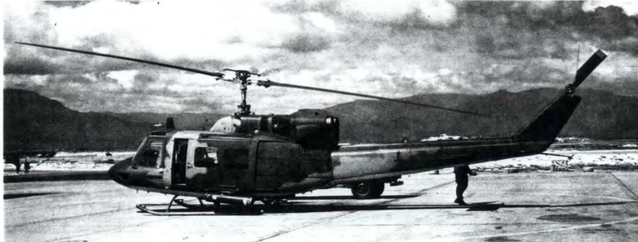
(Above) A twin-engined UH-1N version of the Huey at Cam Ranh Bay in late 1971, carrying LAU-59/B rocket pods, with mini-guns stowed in the cargo cabin. (Photo Tom Hansen.) (Below) An SOG team leaves a "Green Hornet" UH-1N after a mission. This aircraft is equipped with the XM-23 system which utilises M60D machine guns on pintle post mounts. (Photo via Bob Chenoweth.)
