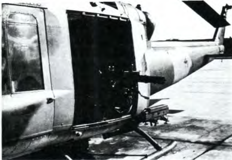
(Above) One of the "Green Hornet" UH-1Ps in February 1971 with the GAU-2B/A mini-guns and later style bomb racks. (Photo Jim Ball.) (Below) One of the original 20th SOS pilots, Maj Tom Garcia (lower left) with a typical SOG team (four indigenous Vietnamese and two US personnel) alongside a "slick" UH-1F. Rope ladders and body armour plates are visible on the cabin floor, and the infantry-type M60s fastened in the doorway have metal rods attached to the barrels to prevent them being fired into the aircraft. (Photo Tom Garcia.)
