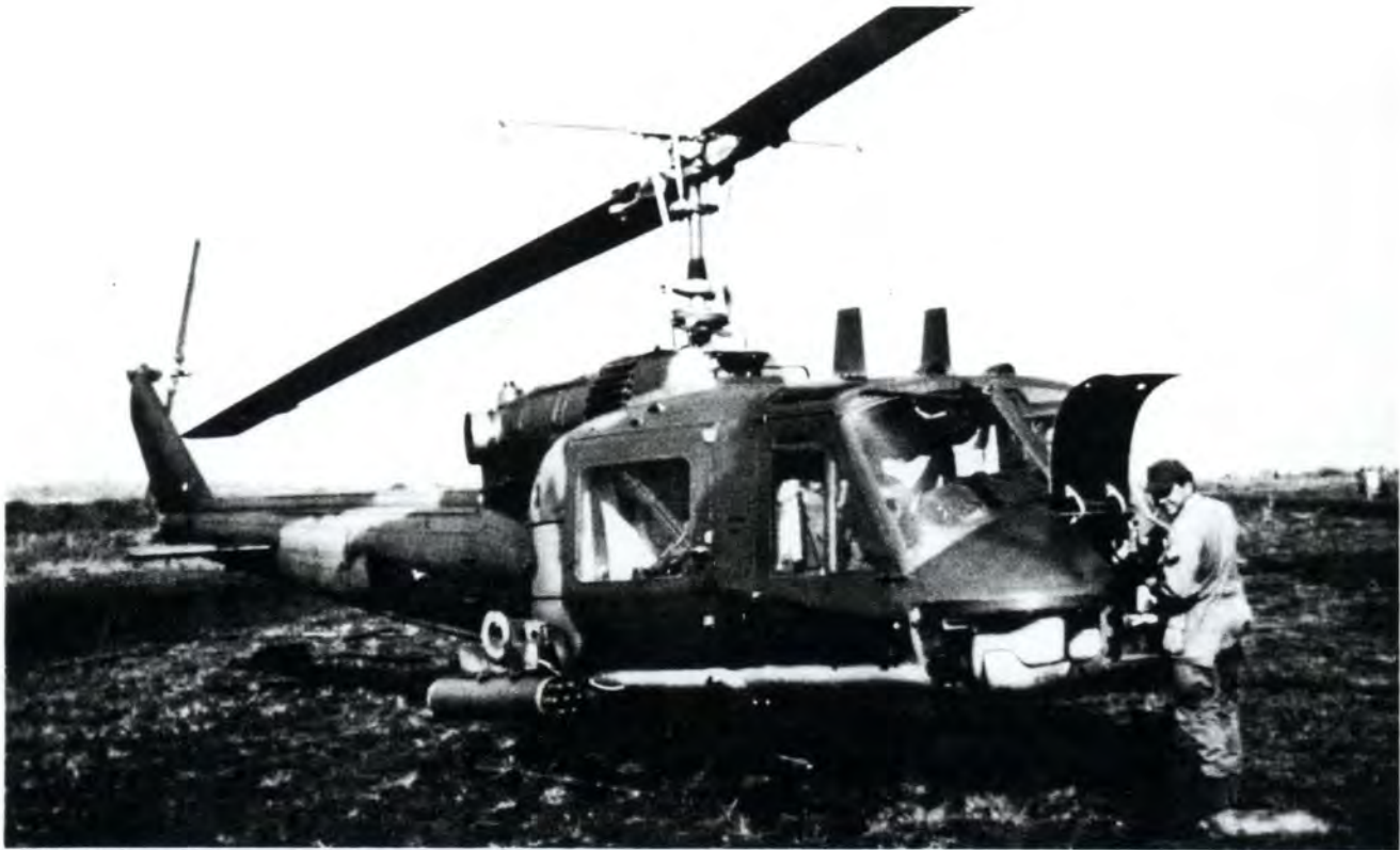
The UH-1P shown in close-up at the foot of the opposite page is here seen receiving further attention from a ground crewman. The rocket pod, stowed mini-gun and dual UHF/VHF antenna are all visible. (Photo via Bob Chenoweth.)
