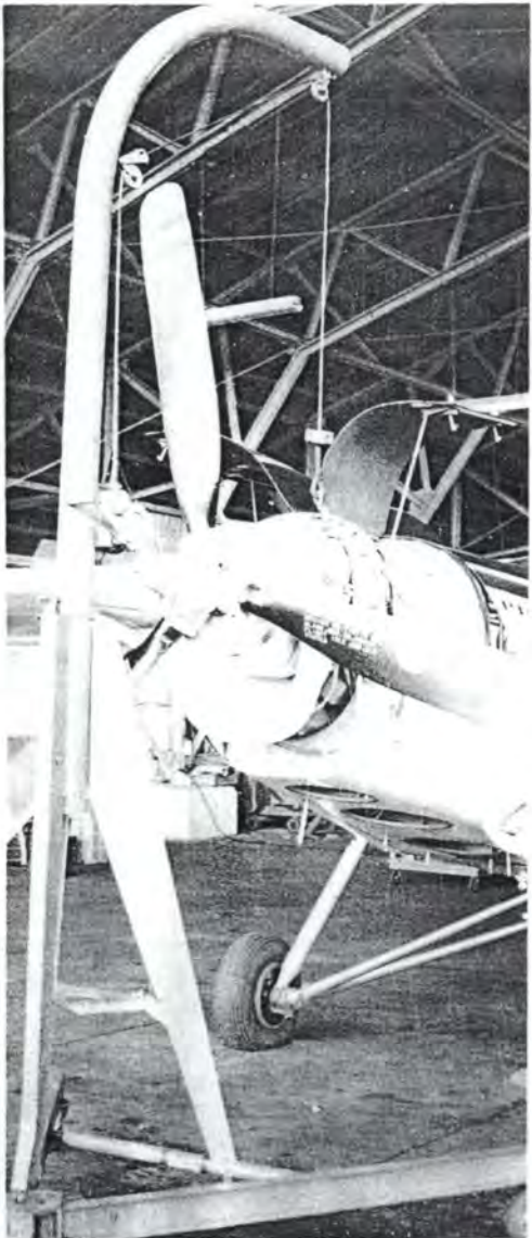
The portable engine hoist being used to change a Garrett TPE 331 turbo-prop engine on a Porter PC-6 plane.
