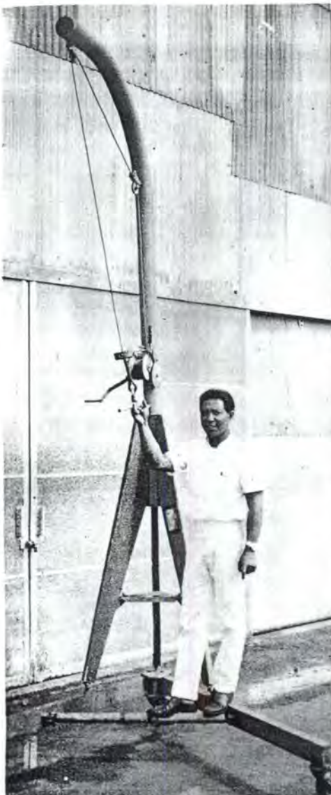
AMD Superintendent F. G. Vizcarra standing on the base of the knock-down engine change hoist he designed.
