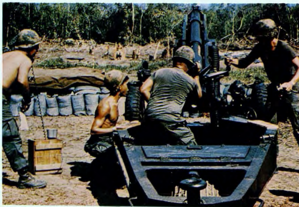
As the gunner checks his aim, another artilleryman prepares to yank the lanyard that will start the 105 mm howitzer's 38-pound high explosive shell on its way.
