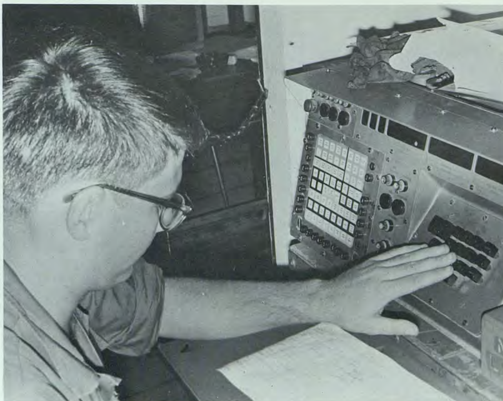
The request for artillery fire has been received and fire direction center (FDC) personnel work to plot the fire mission. An FDC artilleryman used the field artillery digital computer to produce and double check the fire mission data. The information is then radioed to the battery which has been picked to deliver the high explosive support to ground troops in contact with the enemy.
