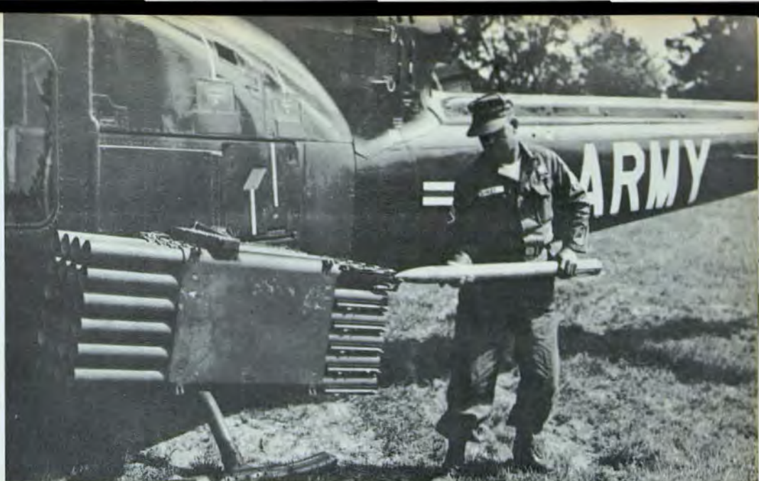
A sergeant involved in test exercise SKY SOLDIER I in 1965 loads a 2.75 inch rocket into the weapons system mounted on an earlier model Huey, the UH-1B.
