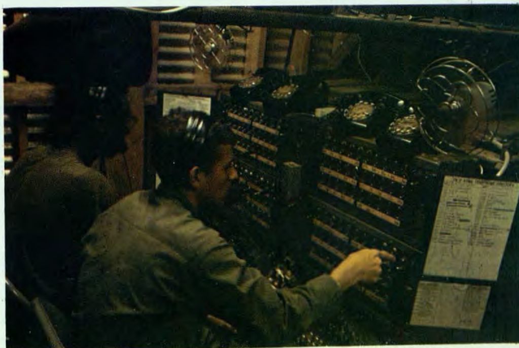
The division headquarters, the three brigade basecamps and some of the Cav's firebases, are also connected by telephone communications. The around-the-clock business of war demands that switchboards (above) be manned constantly. But the bulk of combat communications is carried on the radio waves, from the single platoon radio to what often looks like a small and thin forest of antennas (right) at headquarter areas.
