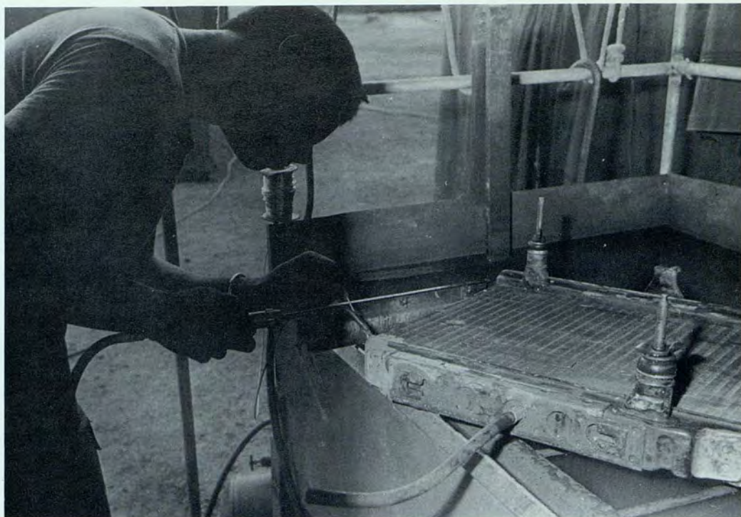
One of the 27th's most important missions is that of keeping more than a thousand division vehicles in working order. Here a mechanic closes a small shrapnel hole in a jeep radiator.
