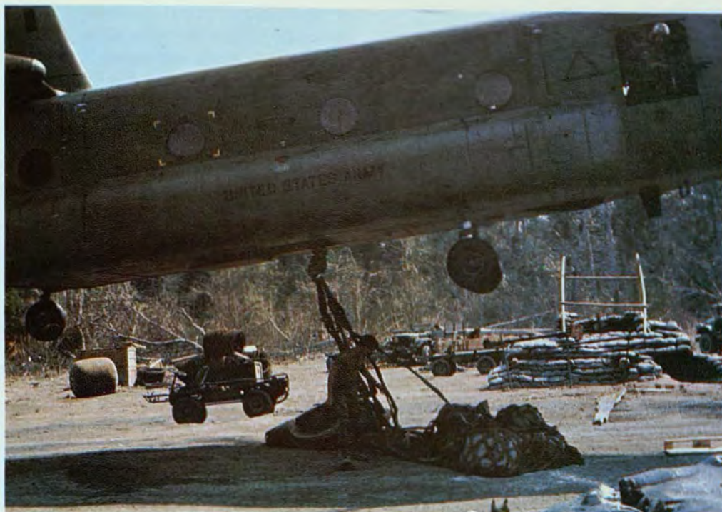
A Redhat, one of the 15th S&S men who rig and hook sling loads for Chinook and Flying Crane transportation, steps away from a load of empty water blivets before they swing free of the ground.
