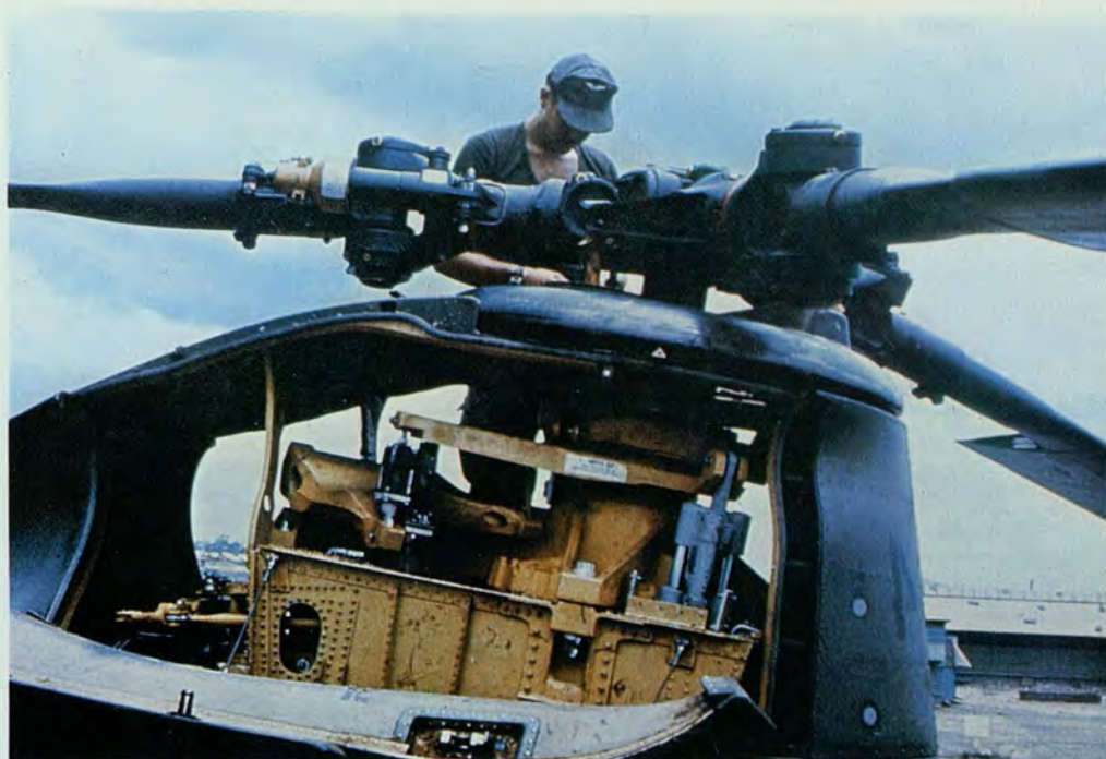
Almost dwarfed by the large tail rotor assembly of a CH-47 Chinook, a mechanic performs the required 100 flying hours inspection and maintenance. Every 1,800 hours of flight, the giant Chinooks are completely torn down and rebuilt, making sure that every part functions perfectly.
