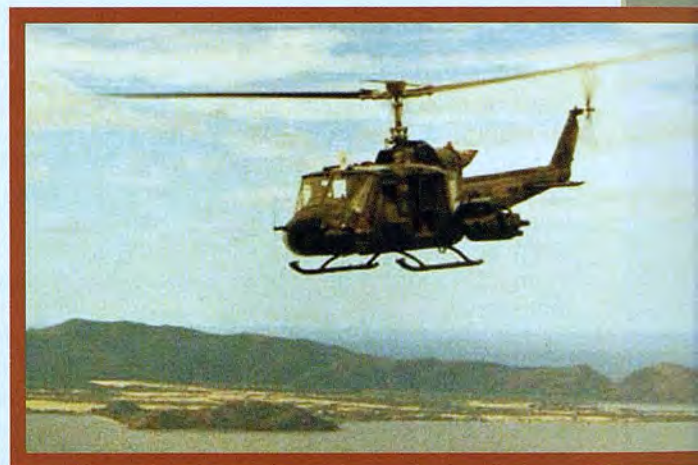
Camouflaged UH-1B with XM-26 TOW armament subsystem.
