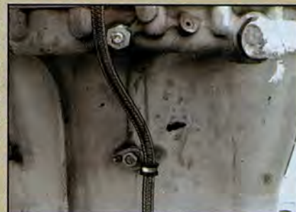
Bullet Hole from Automatic Weapon Damage to Forward Transmission Visible with Cork
