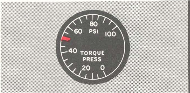
TORQUE PRESSURE 50 PSI Maximum H ONLY
