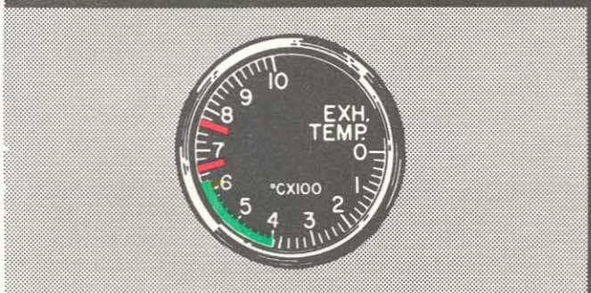
EXHAUST TEMPERATURE T53-L-13A ENGINE 390°C to 610°C Continuous Operation 610°C to 625°C 30 Minute Limit 675°C 5 Second Limit for Starting and Acceleration 760°C Maximum for Starting and Acceleration
