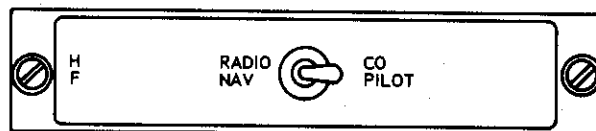
Figure 4-34. HF/COMM Switch Panel
