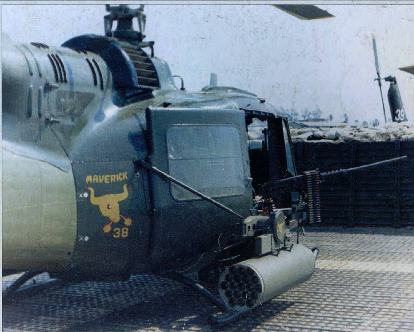
"Maverick 38," a UH-1C gunship with the Third Platoon, 175th Assault Helicopter Company, sits in a revetment at Vinh Long in 1968. The gunship carried two 19-shot 2.75 FFAR pods, a 40 mm M-5 grenade launcher and a .50-caliber machine gun. Photo courtesy of J.F. "Jim" Speirs Jr., a 175th AHC pilot in 1968-69.
