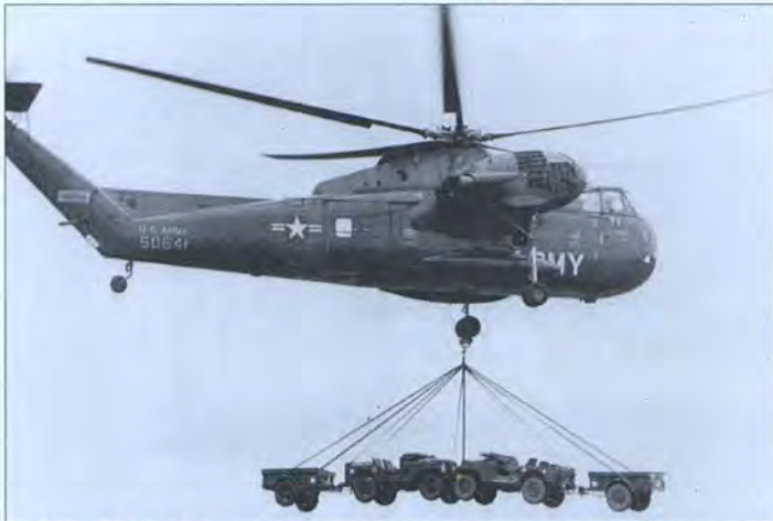
A CH-37 Mojave slingloads two Jeeps and attached trailers. The Mojave was flown in South Vietnam during the early and mid-1960s.
