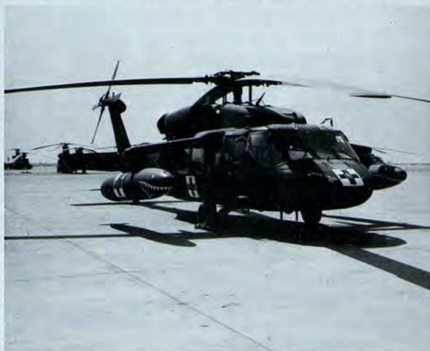
Desert Storm UH60 equipped for long range self-deployment from Germany to Saudi Arabia.
