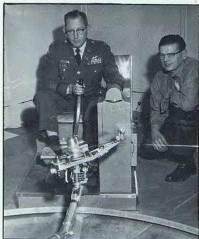
LEFT: Colonel E.P. Fleming, Jr., Fort Wolters commander and Primary Helicopter School commandant, tests the latest device that can be used in training helicopter student pilots, as P.C. Jacobs (right), inventor of the training aid and vice president of the Jaycopter Corp. Ltd. of Canada, looks on. Called the Jaycopter Demonstrator-Trainer (JDT), it is a miniature captive helicopter connected to the controls by hydraulic lines. Cyclic control movements are resolved into electronic impulses which are fed into the operator's instrument panel. Present plans call for experimental use of the JDT with a limited number of helicopter students to determine its training effectiveness. BELOW: Lt Gen Robert W. Colglazier, Fourth Army CG, inspects members of the Fort Wolters honor guard during ceremonies January 11 at the Primary Helicopter School. The occasion for the visit was Gen. Colglazier's farewell prior to his coming retirement.
