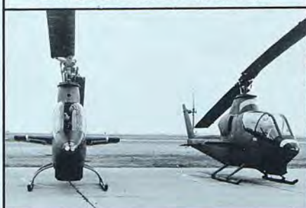
The first of two pre-production models of the HueyCobra is shown at the left, with Bell's prototype at the right. Curved landing gear, wider turret, slightly larger wings, and fixed steps for the pilot and gunner are noticeable changes. Bell has an Army production order for 110 HueyCobras, with the first deliveries of the world's first fully-integrated weapons helicopter next spring.
