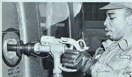
Automatic Shut-Off Nozzle and conventional refueling nipple during refueling operation
