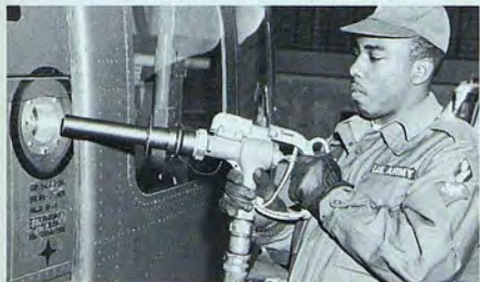
Automatic Shut-Off Nozzle attached to conventional refueling nipple
