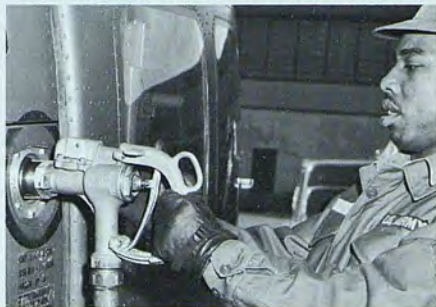
Automatic Shut-Off Nozzle inserted into Adapter mouth and ready for refueling
