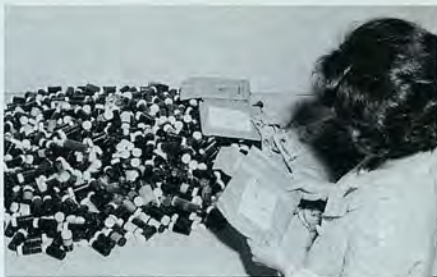
Michiko Takahara, a Ryukyuan employee at the 2d Logistical Command's spectrometric oil analysis lab in Okinawa, opens mailbag containing oil sample from aviation companies in Vietnam. The lab analysis monitors the metal particles in the oil to detect engine trouble in advance. (★Exclusive)
