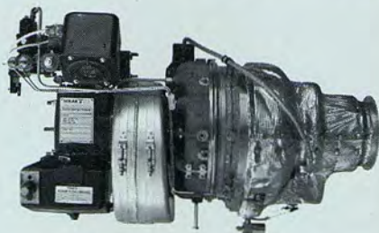
Titan APU—weight 70 lbs, over-all length 26 inches
