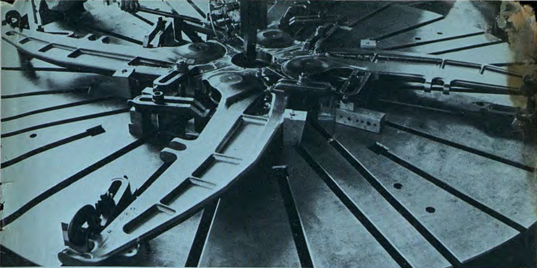
ABOVE: MACHINING A TITANIUM AAFSS ROTOR HUB
