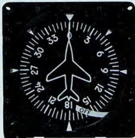
New ARC G-112A electric directional gyro gives you easy to read vertical card presentation and its 12°/hour drift rate exceeds TSO specifications. It only weighs in at 3 lbs. and you can mount it in panels inclined up to 10° without affecting specs.
