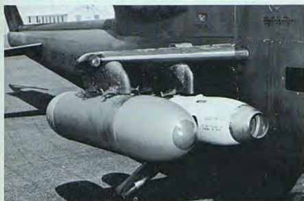
XM-159 with nose fairing (left) and XM-18 Podded Mini-Gun (right)
