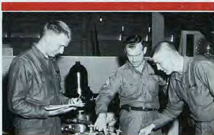
68E20 (Propeller and Rotor) Students, check out propeller cam operation with a hydraulic tester at ATMD, Fort Eustis, Virginia.
