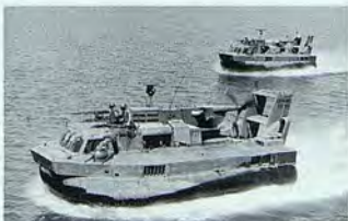
BUFFALO — Textron's Bell Aerosystems Company recently announced the delivery of three Amphibious Air Cushion Vehicles (ACV) to the U.S. Army. The armed and armored Bell ACV's are capable of 30-mph speeds and can perform a variety of missions, including amphibious assaults, search and rescue, high-speed personnel transportation, or patrol and logistic support over land, water, mud, snow, and marsh. The Assault Air Cushion Vehicles (AACV) are equipped with a .50 caliber machine gun in each of the two roof turrets and a 7.62 mm machine gun in each of the two rear cabin windows. Also aboard is a 40 mm M5 port side grapple launcher capable of firing 225-330 rounds per minute.
