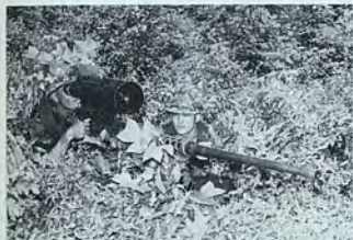
PORT MONMOUTH — The latest tactical night vision device, which will enable U.S. fighting men in Vietnam to draw a clear, bright beam on the enemy in the dark night, using the faint glow of starlight were made public recently by the U.S. Army. The device, which range from hand-held straight scopes to larger night vision goggles for crew-served weapons and more distant viewing, were developed by the Night Vision Laboratory of the Army Electronics Command (ECOM), a major element of the Army Materiel Command, and many of them are now in use in South Vietnam.
