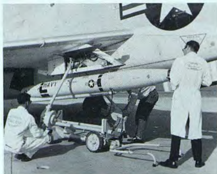
This Beech AQM-37A target missile is used as the test-bed for the first U.S. hybrid rocket propulsion system, developed by United Technology Center, Division of United Aircraft Corporation. During first tests the missile was sent to altitudes up to 80,000 feet, to speeds in excess of 2,000 mph and demonstrated its maneuverability at supersonic speeds—exactly as planned.
