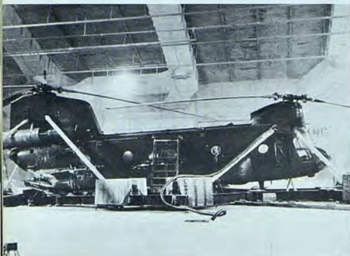
ELGIN AFB, FLA. — The U.S. Army's newest model Chinook medium transport helicopter, the Boeing-built CH-47C, recently completed environmental testing in the Air Force's climatic laboratory at Elgin AFB. Shown here in the lab's main test chamber, the "C" model Chinook was subjected to temperature variances ranging from -65°F to 125°F. Later this year, the "C" model Chinook is scheduled for hot weather suitability testing near Yuma, Arizona, and a high altitude evaluation at Pike's Peak, Colorado. (Boeing)
