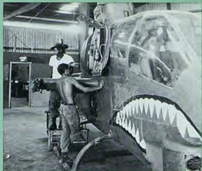
CU CHI, VIETNAM — The shark-like appearance of a Cobra is quite evident in this behind-the-scenes maintenance effort. Here, three crewmen use a winch to set the Cobra transmission in place. Work with heavy equipment is a daily task for Echo Company men of the 725th Maintenance Battalion, 25th Infantry Division.
