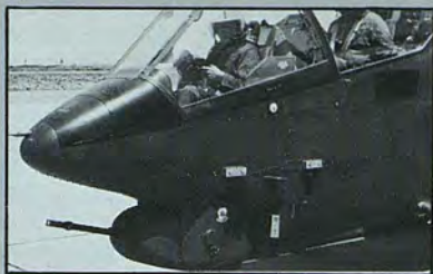
UNDER TEST — An AH-1G HueyCobra equipped with an XM-140 30mm gun is currently undergoing Army evaluation at the Mojave, Calif. Test Range. Capable of a 425 shot per minute rate of fire, the XM-140 is an electrically-powered single barrel automatic gun destined for use against light armored vehicles and emplacements. LTC Dean Wright of the AAWS Office, AVSCOM, and Bell test pilot R. G. Kjellander are shown in the co-pilot/gunner and pilot seats. (Bell)
