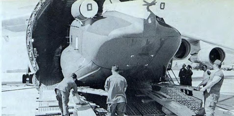
*The C5's loading ramp must be modified so that CH-47 clears ceiling of cargo compartment.*
