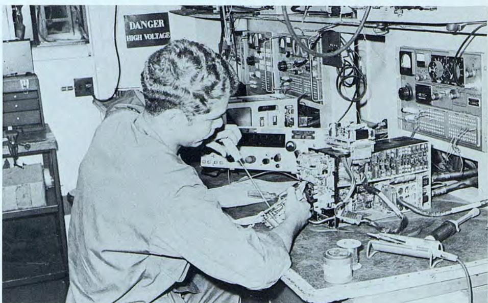
*A doppler technician of the 317th LEM Co. replaces a module in a memory storage unit, a part of the computer in the AN/ASN-64 Doppler Radar System.*
