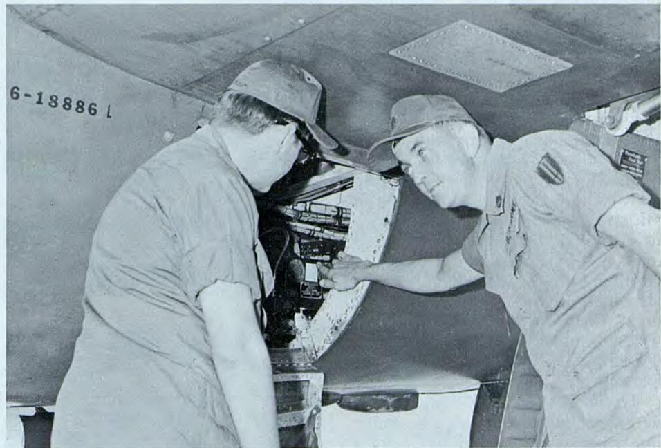
*A SLAR repairman trouble shooting a module on test set AN/USM-187 the only such test set in-country.*
