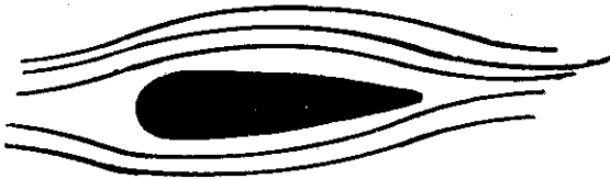
NORMAL AIRFLOW PRODUCING LIFT
