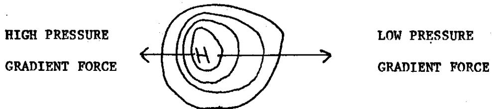
The pressure gradient force is the first physical force that affects the movement of air. The speed of air movement, or winds is dependent upon the intensity of the pressure gradient force.
