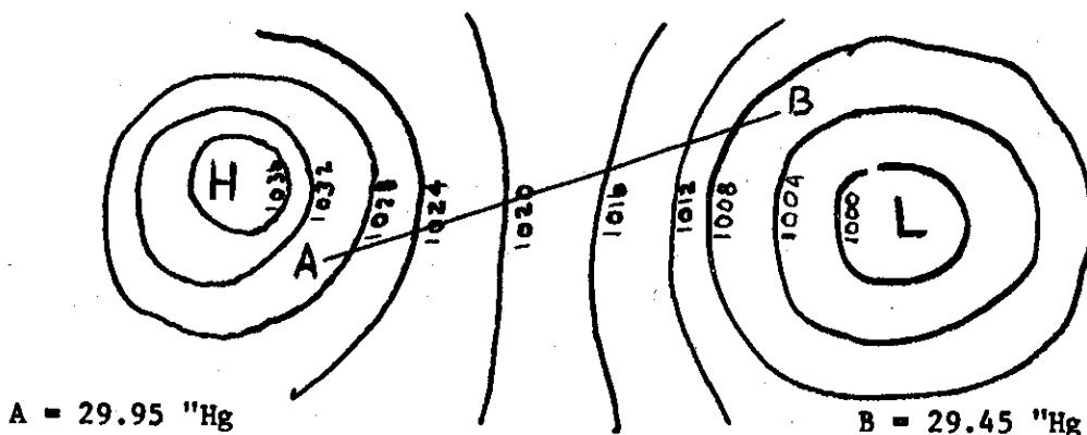
Flying from an area of higher pressure to an area of lower pressure, an aircraft will be lower than the indicated altitude unless the altimeter setting is corrected to the new area.
