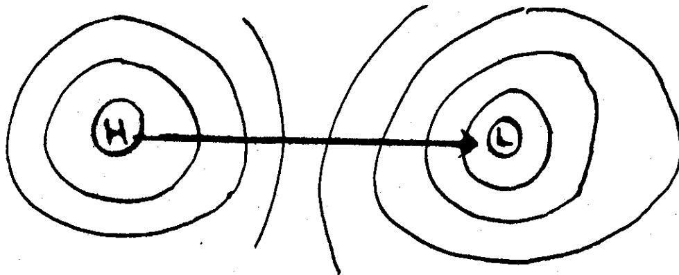
A high pressure area (H) is formed by an isobaric pattern in which the highest pressure exists at the center. It is also called anti-cyclone. In a low pressure area, the lowest pressure is found at the center and it is identified by the letter L. A low is often referred to as a cyclone.
