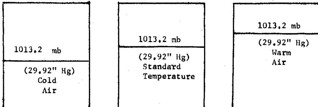
A specific millibar level will be higher than standard in warm air, and lower than standard in cold air.
