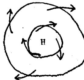
Frictional force is generally effective at altitudes to 2000 ft above the surface. Above this level, winds would tend to be parallel to the isobars.
