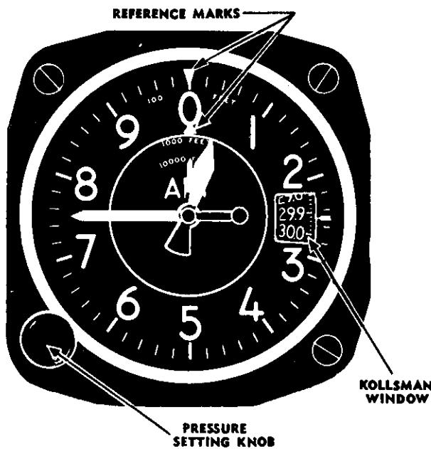
In the above diagram, the altimeter indicates that field elevation is 750 MSL ft.
