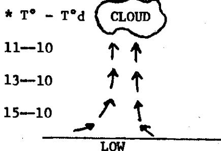
Rising air cools causing its temperature to approach the dew point. Condensation occurs and clouds develop.
