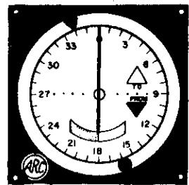
8. An aircraft is tracking westbound on V-12. After tuning to station C and setting the course selector, the pilot observes the course indicator as shown. The aircraft has:
