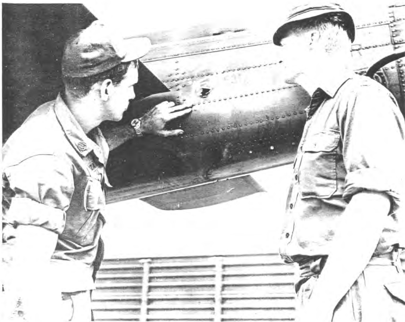
Ldg Seaman Tudor and a US Army maintainer inspect a large calibre bullet hole in the tail boom of a Huey. (ANAM)
