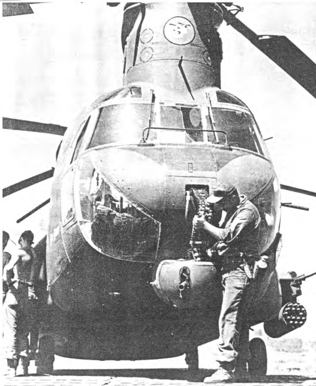
In 1966 1st Air Cav Div evaluated 3 armed CH-47 Chinooks in combat. They mounted 40mm M-5 grenade launchers, 2.75 FFAR's, 20mm cannon, and five .50 cal. window mounted machine guns.
