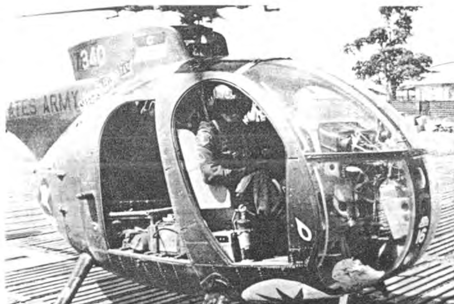
Hugh Mills in "Miss Clawd IV." External power receptacle is immediately behind fire extinguisher. Note position of "Darkhorse" emblem on front of Loach.
