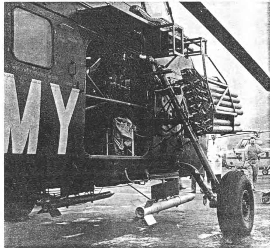
Armed H-34 carried twin 20mm cannon, twin 50 caliber MG, 40 2.5 FFAR, twin 30 cal MG (window mounted), 4 30 cal. MG (tracer firing for rocket aiming), 2 5" Tiny Tim Rockets, and one 50 cal MG in window mount.
