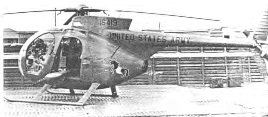
Another of Mills' mounts. (See cover painting for Darkhorse markings colors.) Loaches carried 2,000 rounds for minigun, which could be set to fire at 2,000 or 4,000 rounds per minute. (Hugh Mills)
