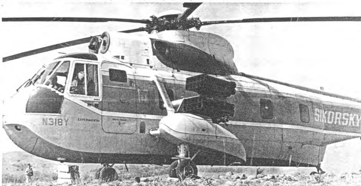
Sikorsky SH-3 Sea King mounting 40 4.5" rocket tubes, capable of elevation and depression. (Sikorsky)
