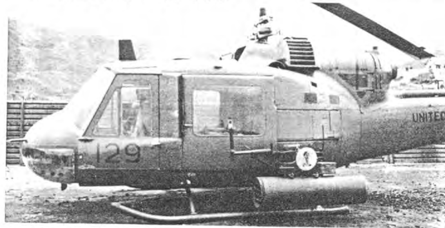
UH-1C flown by WO/1 Bill Gambriel, Vietnam 1969-70. (see color illustration in center section) When these pictures were taken it had just had windscreen and overhead greenhouse panels replaced, due to VC bullet damage. It was later destroyed in combat. (Bill Gambriel)
