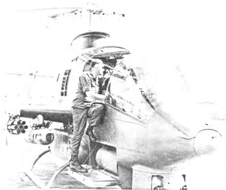
Preliminary instruction in preflight of the AH-1G armed with 20mm Vulcan cannon, at Cobra Transition School, Vung Tau, Vietnam. Note: Installation of the XM-18 Pod on right inboard, and M-35 on left inboard is unusual.
