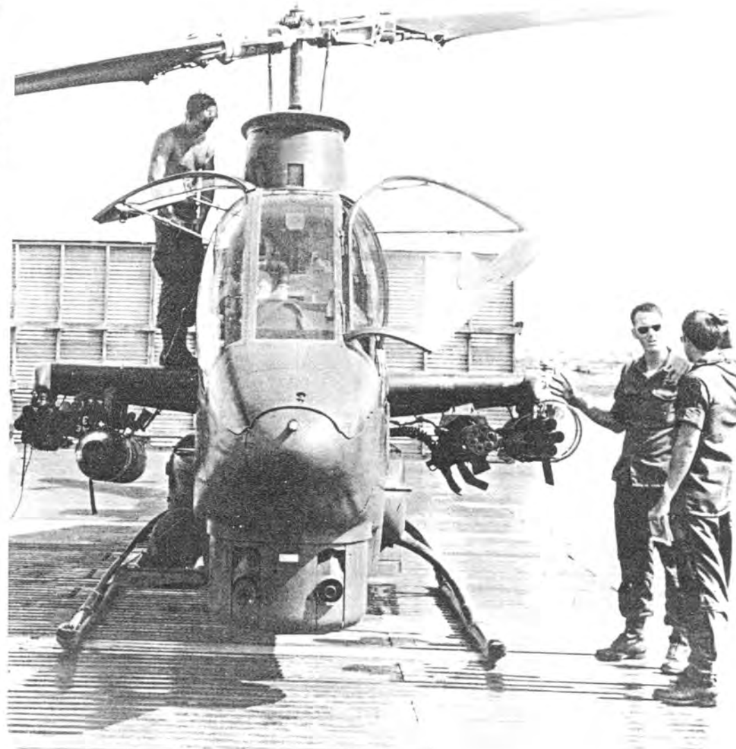
Preliminary instruction in preflight of the AH-1G armed with 20mm Vulcan cannon, at Cobra Transition School, Vung Tau, Vietnam. Note: Installation of the XM-18 Pod on right inboard, and M-35 on left inboard is unusual.
