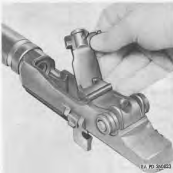
Figure 35. Removal and installation of bolt assembly.
