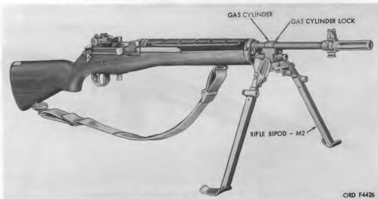
Figure 4. 7.62-mm rifle M14 with bipod installed - right front view.
