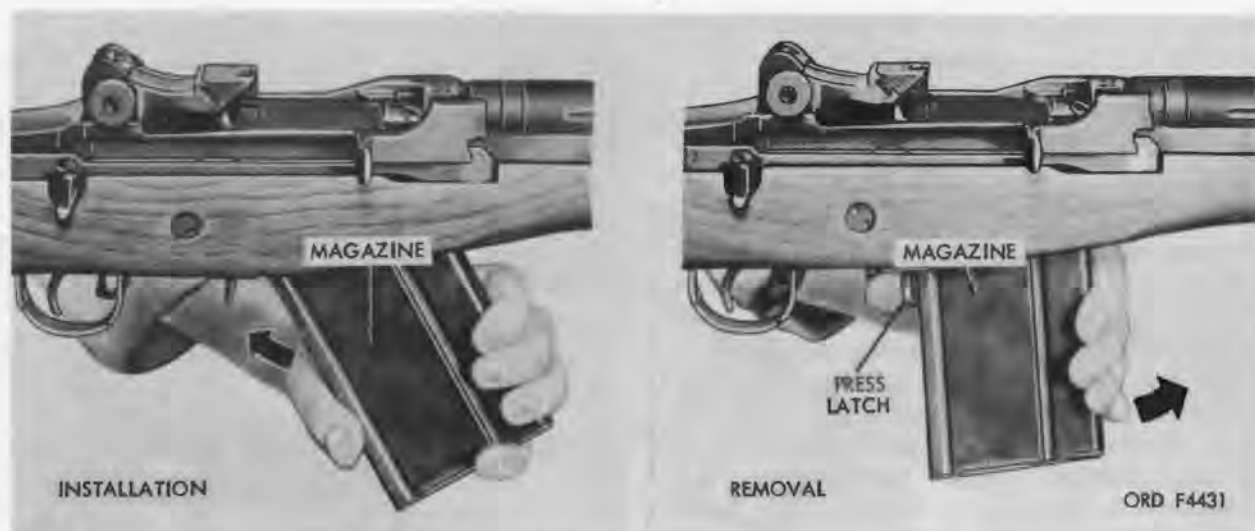
Figure 17. Installation and removal of the magazine.
