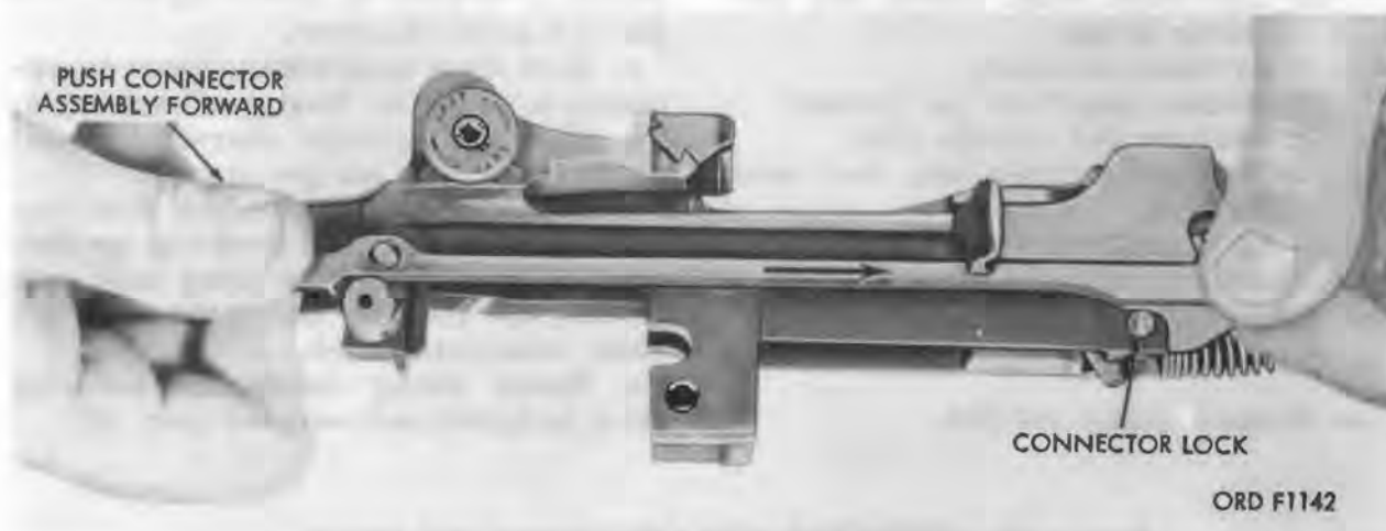
Figure 31. Disengaging of connector assembly.
