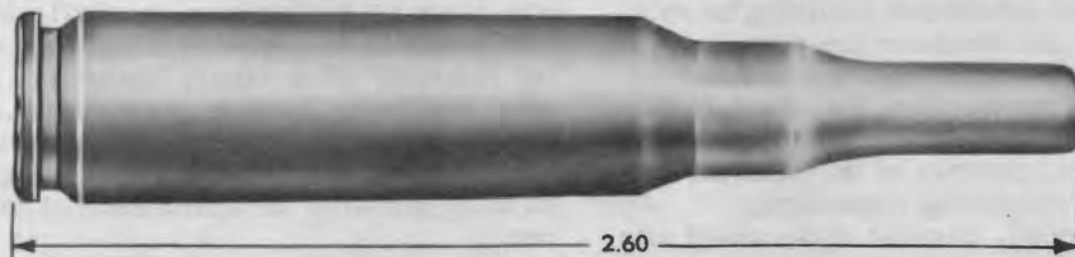
CARTRIDGE, 7.62 MILLIMETER BLANK: NATO, XM82
