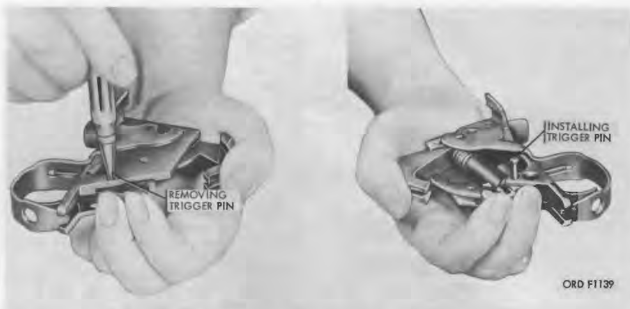
Figure 28. Removing and installing trigger pin 7791367.
