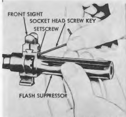
A. REMOVAL AND INSTALLATION OF FLASH SUPPRESSOR NUT LOCKING SETSCREW
