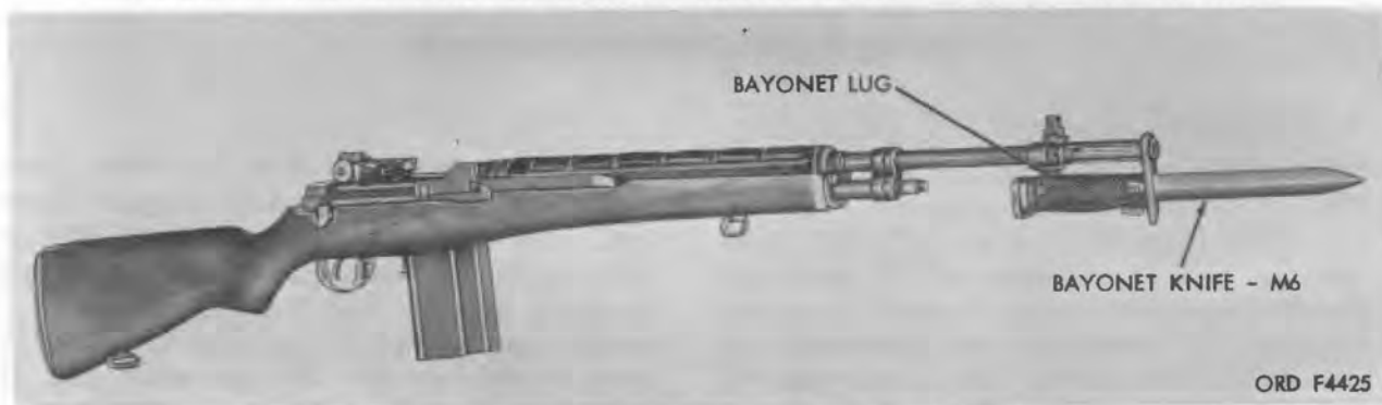
Figure 3. 7.62-mm rifle M14 with bayonet-knife M6 - right front view.
