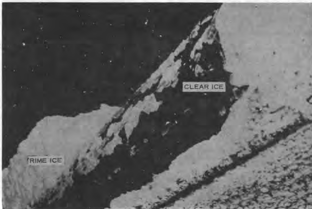
Figure 9-2. Formation of clear (glaze) and rime ice on aircraft wing.
