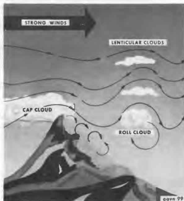
Figure 4-37. Schematic diagram showing airflow in a mountain wave.
