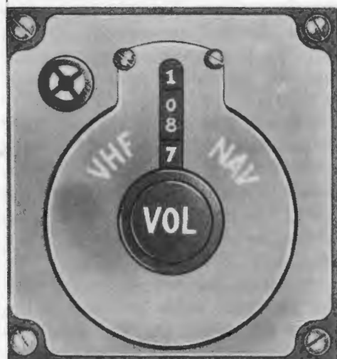
(A) GLIDESLOPE CONTROL PANEL.
