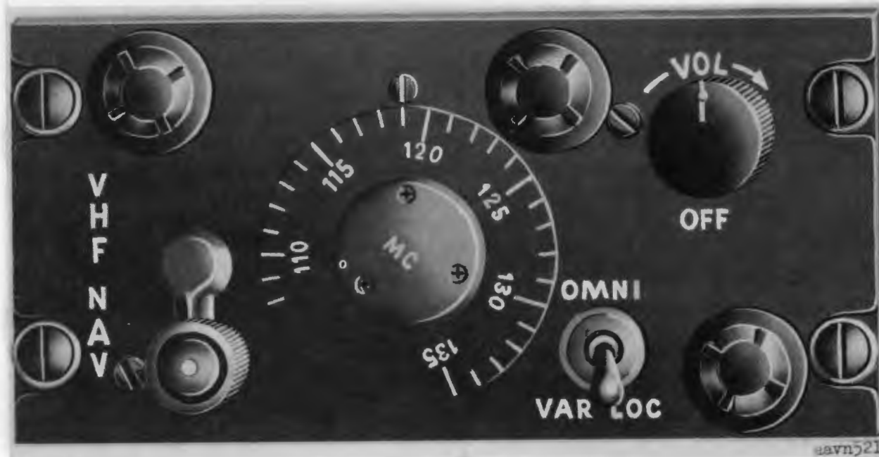
Figure 10-2. ARN-30A receiver control panel.
