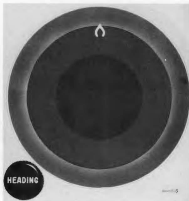
Figure 17-9. Heading marker and heading knob.
