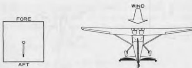
Figure 17. Stick position for taxiing, headwind.
