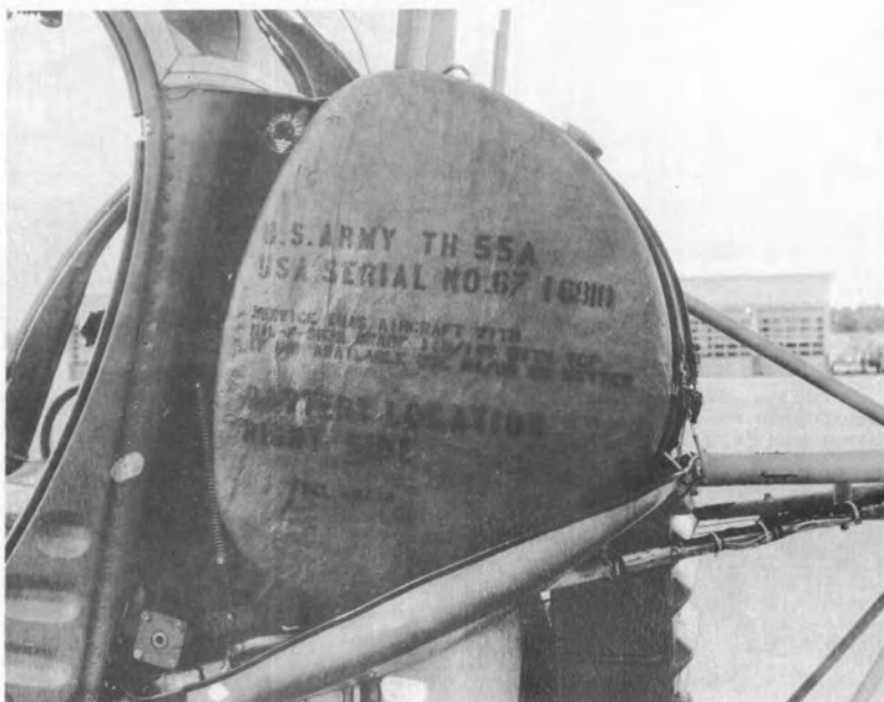
Fuel Tank - Fibreglass Wrapped for Safety (fig. 2-3)
