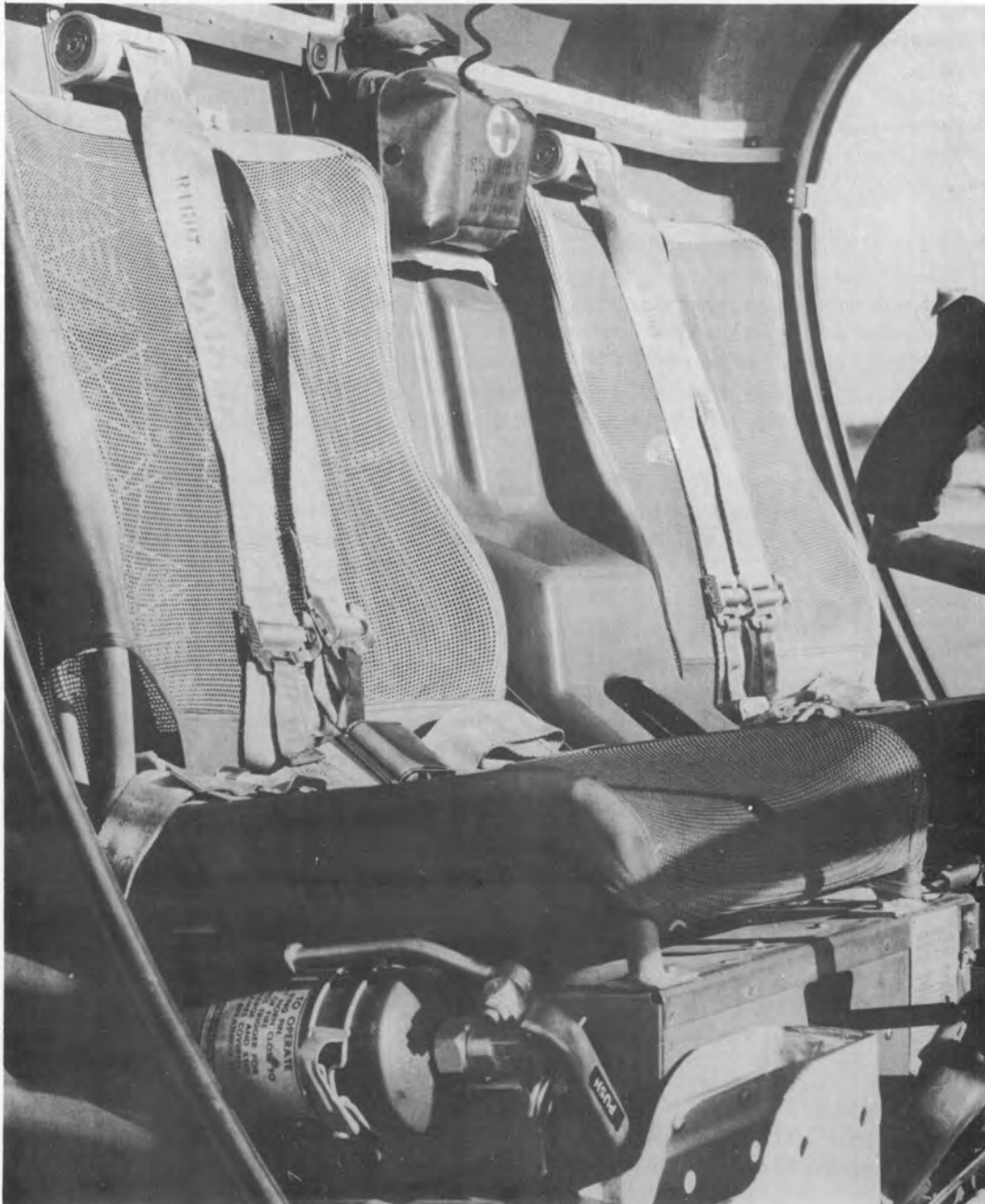
Cockpit View Shows the Location of the Fire Extinguisher, Safety Kit and the Seat Belt-Shoulder Harness Installation: (fig. 2-16)
