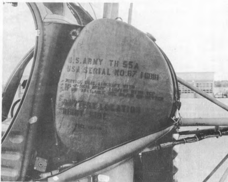
Fuel Tank - Fibreglass Wrapped for Safety (fig. 2-3)
