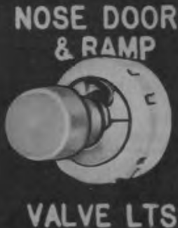
Figure 6-6. Nose door and ramp manual override control light switch
