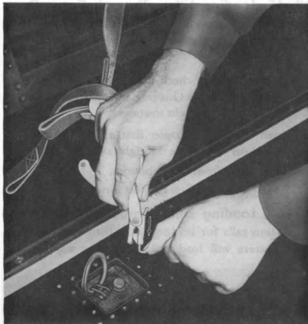
Figure 13-47. Press clip release to open clamp jaws
