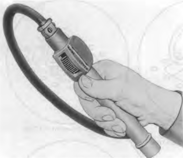
Figure 13-20. Traverse hoist winch control switch and grip
