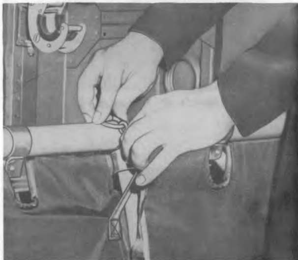
Figure 13-32. Securing folded seat with stowage strap
