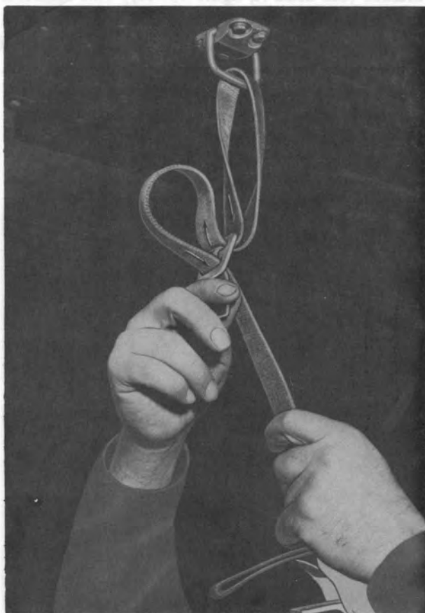
Figure 13-46. Insert strap and through strap buckle
