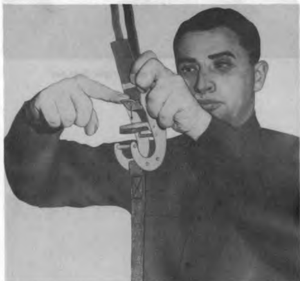
Figure 13-49. Press cam down opening bracket
