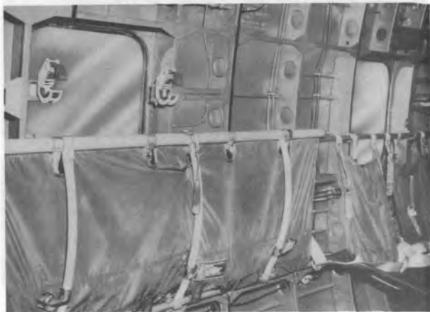
Figure 13-33. Three-man seat folded and secured in place
