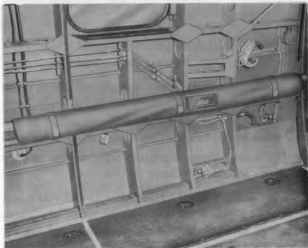
Figure 13-36. Troop seat rolled and stowed
