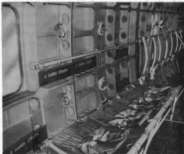
Figure 13-35. Seat back folded on seat
