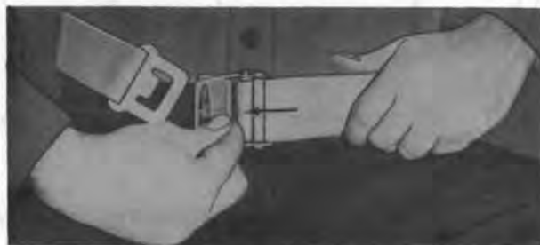
Figure 13-42. Releasing safety belt by lifting on buckle lever on left side of buckle
