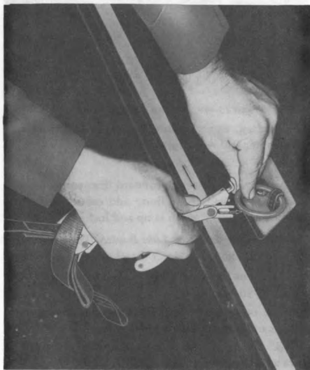
Figure 13-48. Insert tie-down ring into clamp jaws
