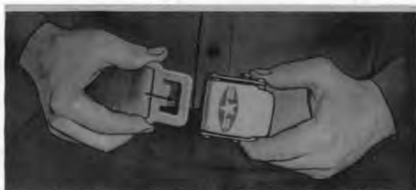
Figure 13-40. Inserting engaging bar into safety belt buckle
