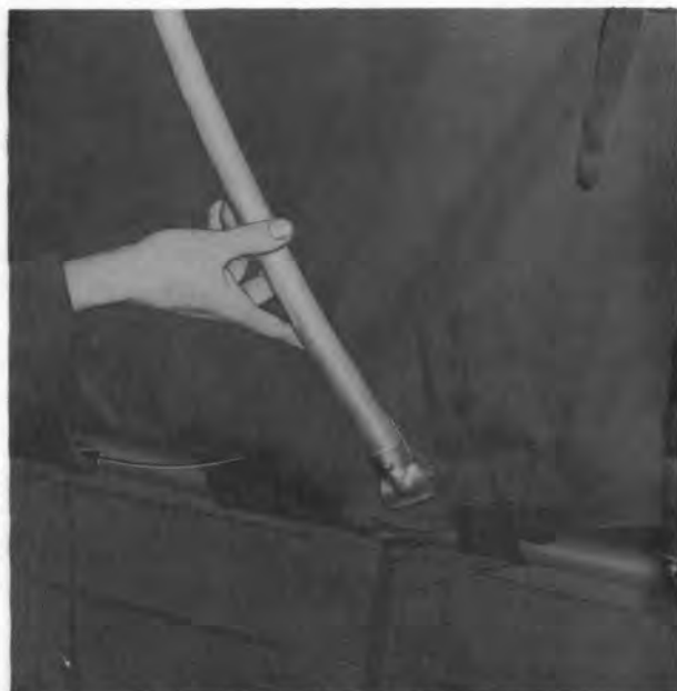
Figure 13-25. Inboard end of seat spreader
