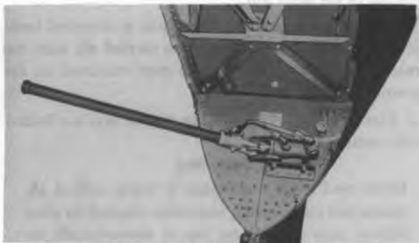
Figure 6-13. Pylon fold valve selector and pump lever
