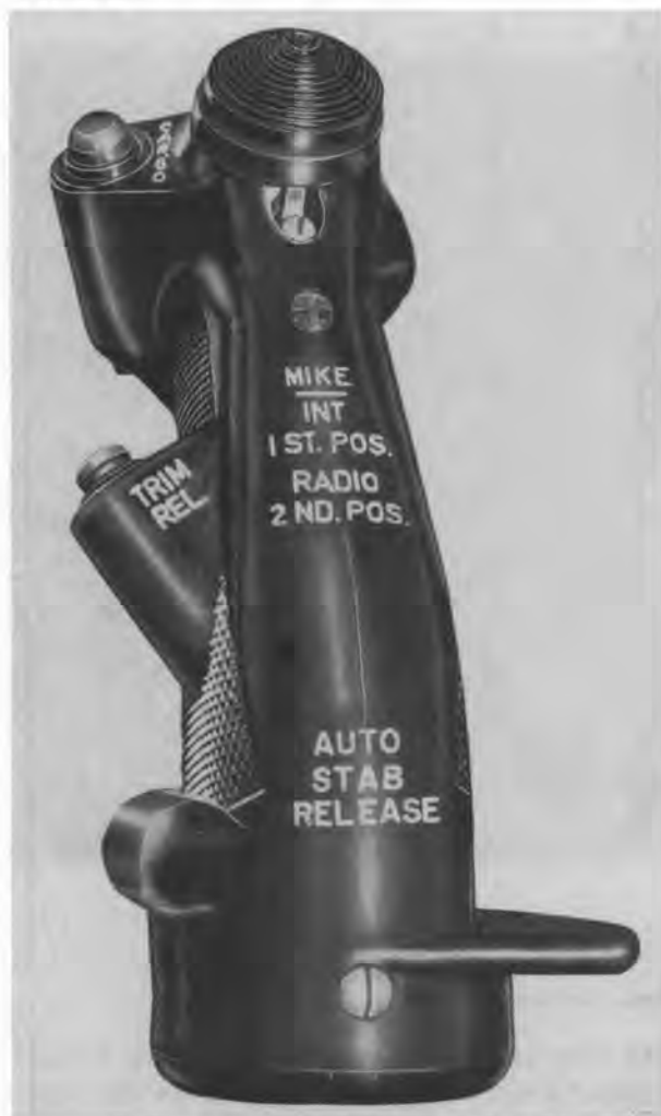
Figure 2-25. Cyclic stick grip (typical)
