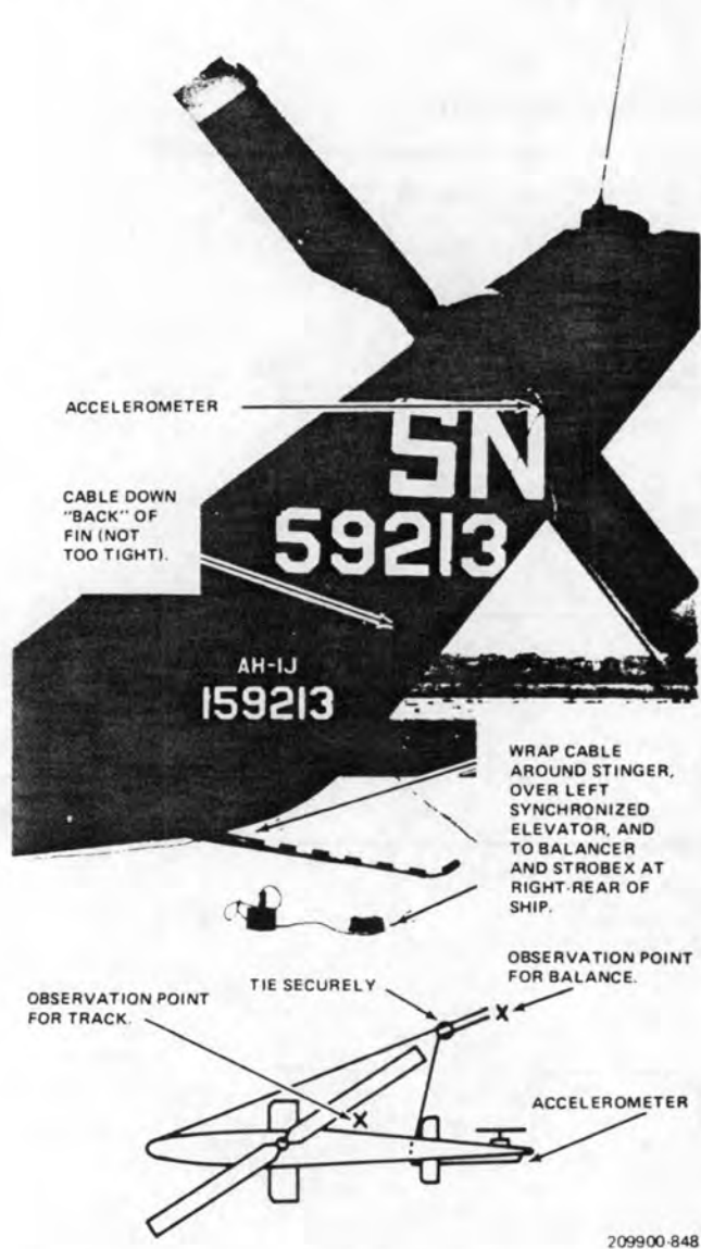
Figure 5-115. Accelerometer Cable Installation (Typical)
