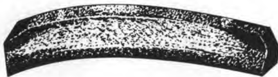
Acceptable wear pattern on pinion View H
