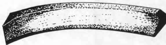
Desired wear pattern on pinion View A
