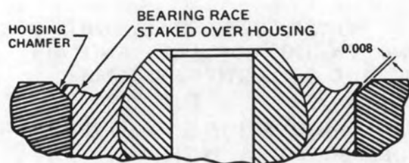
DETAIL B PREGROOVED BEARING (TYPICAL)
