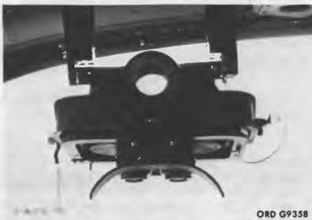
Figure 6-28. M22 Guided missile — gunner's sight, stowed
