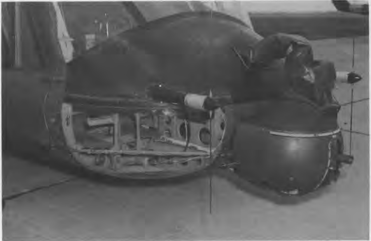
Figure 6-30. M5 Grenade launcher — 40 millimeter grenade launcher installed on UH-1B
