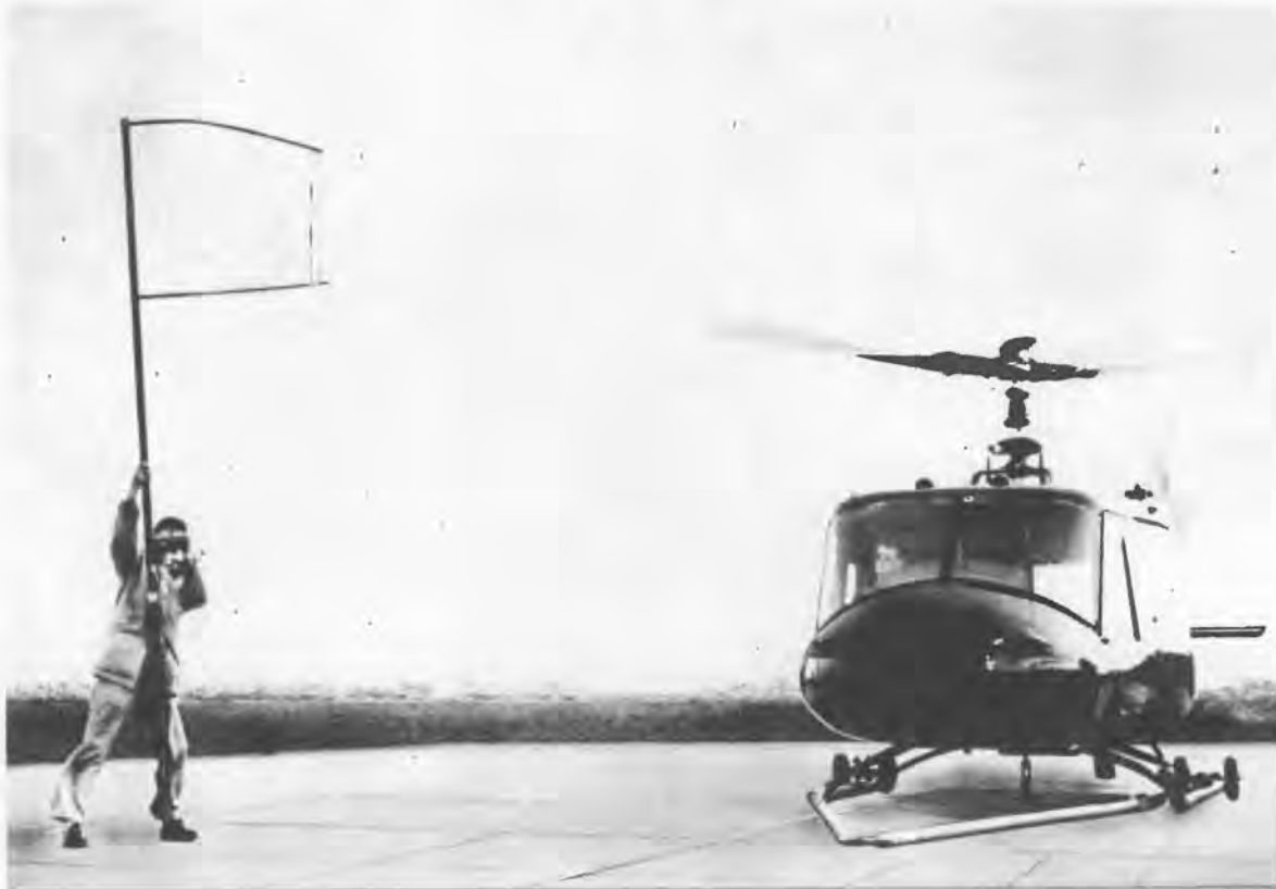
Figure 8-11. Tracking main rotor blades (UH-1B Serial No. 60-3546 thru 64-14100)
