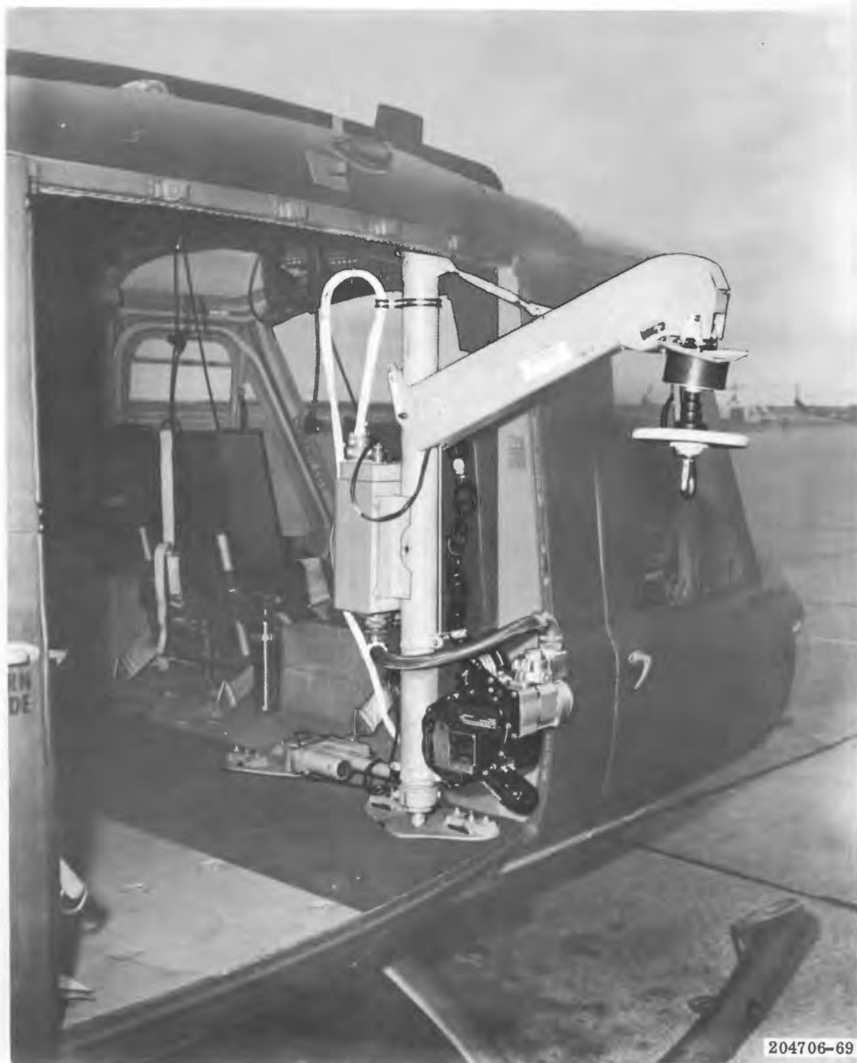
Figure 4-8A. Internal rescue hoist — UH-1B and UH-1C
