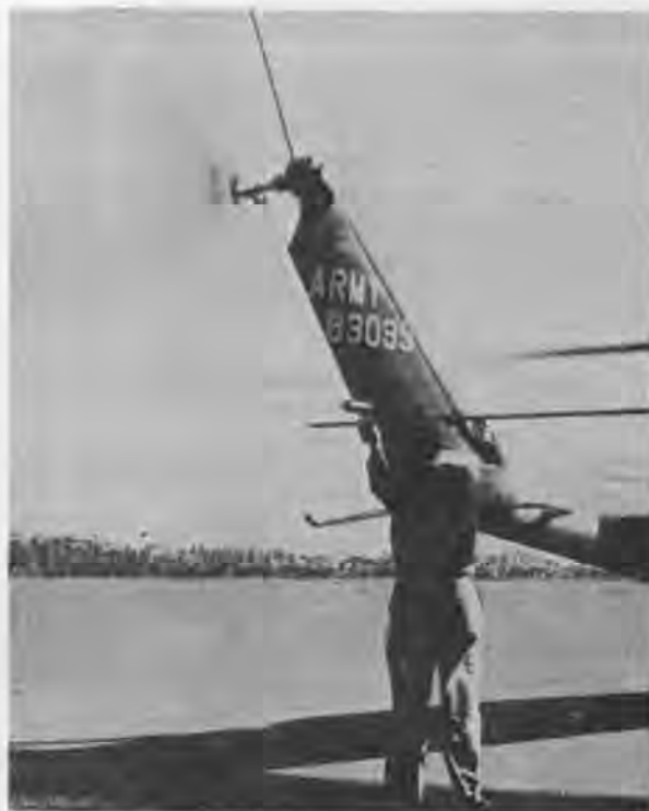
Figure 8-40. Tracking tail rotor blades (UH-1B Serial No. 64-14101 and subsequent)
