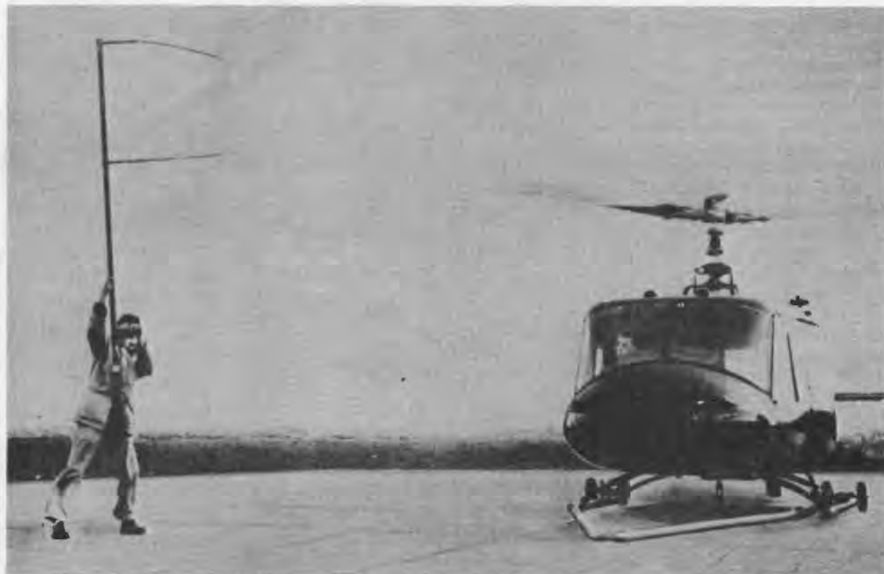
Figure 8-23. Tracking main rotor blades (UH-1B Serial No. 64-14101 and subsequent)
