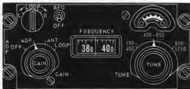
Figure 5-16A. Direction finder control panel — C6899/ARN-83
