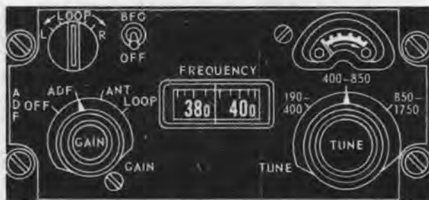
Figure 5-16A. Direction finder control panel — C6899/ARN-83
