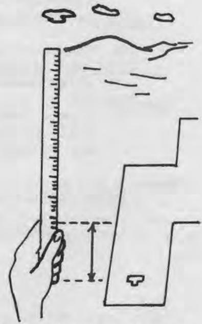
This picture tells me I am too high. The panel has moved further away from the horizon. I need to reduce power.
