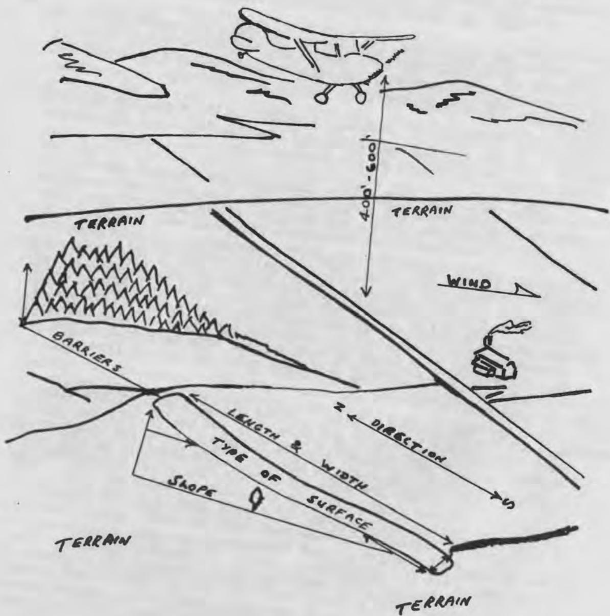
3. The best terrain. The pilot determines the best forced landing terrain around the strip and its relation to the strip. This may be a field, a road or any type of terrain he considers safe for a forced landing.
