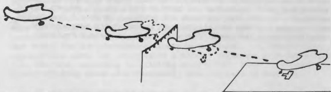
Avoid the tendency to raise the nose as the aircraft nears the barrier.
