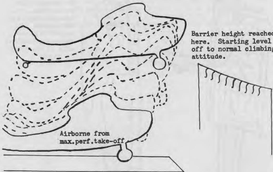
The barrier take-off is begun with the maximum performance take-off. As the aircraft becomes airborne, the nose is raised in a smooth continuous movement and the acceleration is used to gain altitude, while maintaining a constant ground speed. As soon as barrier height is reached, the nose is lowered immediately to normal climbing attitude and the aircraft is allowed to accelerate to climbing airspeed. Rough usage of controls must be avoided.
