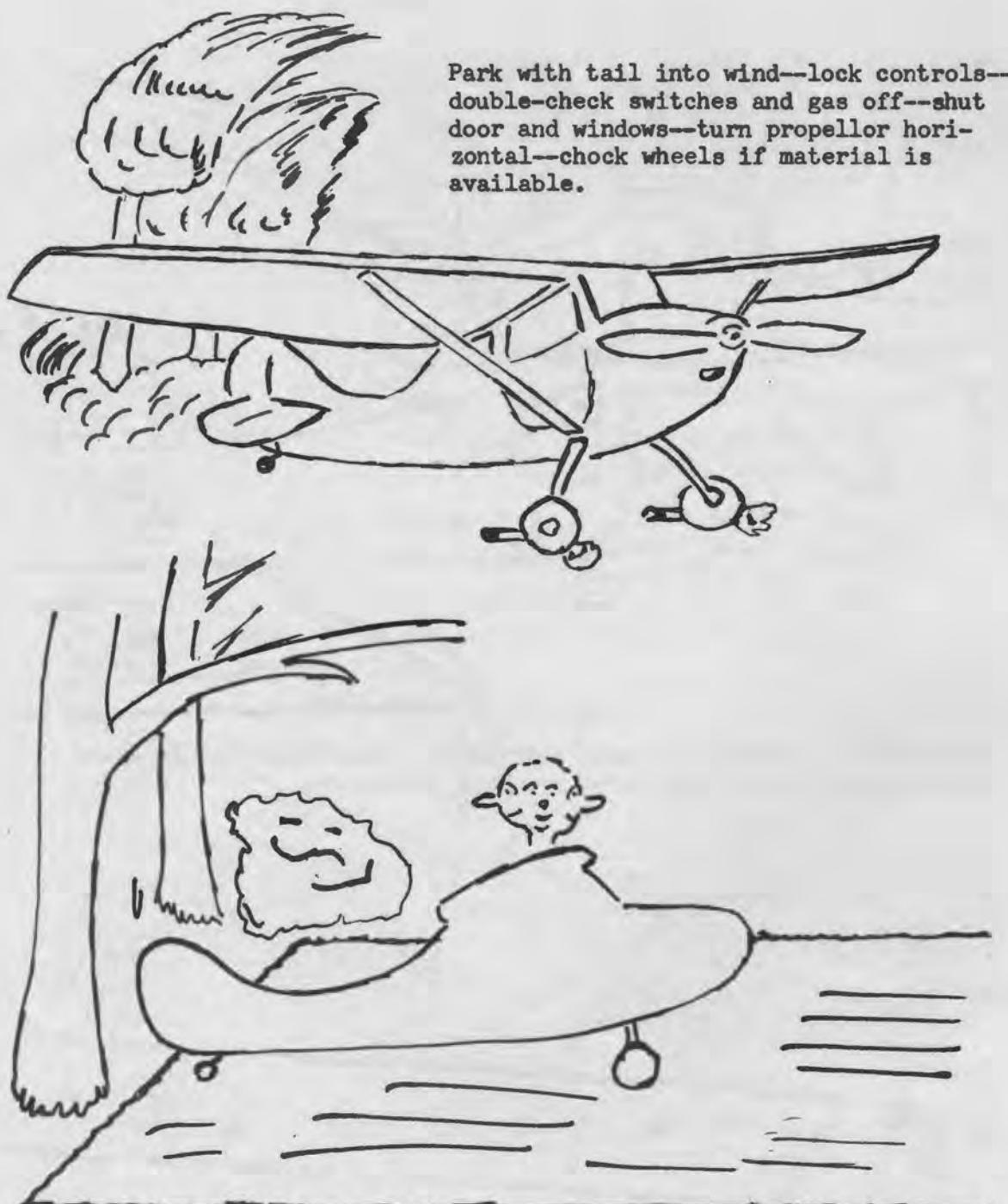
Park with tail into wind--lock controls--double-check switches and gas off--shut door and windows--turn propellor horizontal--chock wheels if material is available.
