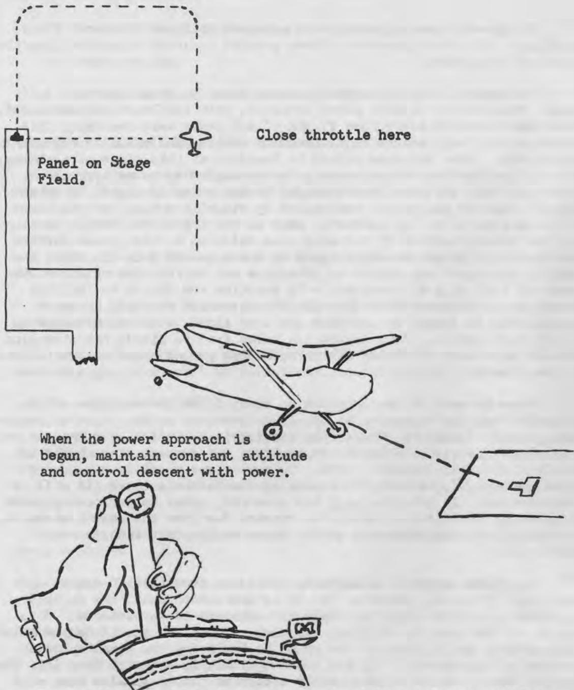
The throttle should be held with the hand in a relaxed position, braced so that the throttle may be squeezed forward and aft. The above illustration shows one method. Students should not hold the throttle in such a manner that sudden, full power application will catch their fingers between the throttle and mixture control.
