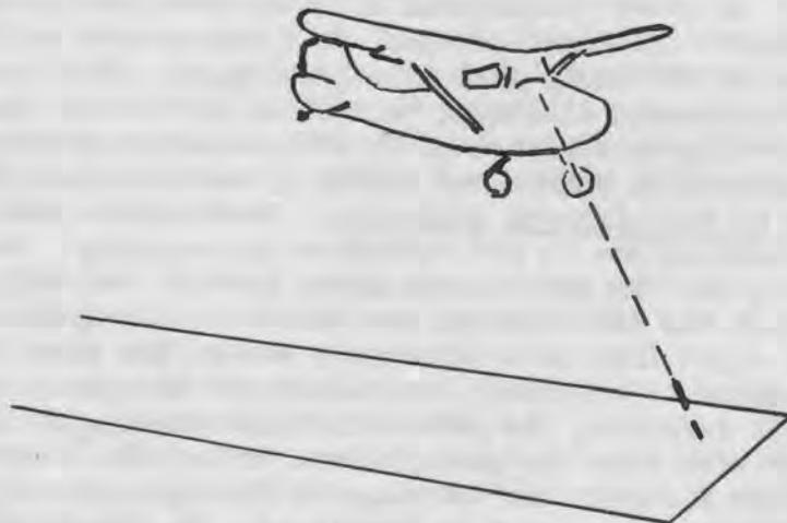
As the aircraft moves along the strip, during the low reconnaissance, the pilot inspects the entire surface of the strip for hazards to the ground roll of the aircraft. As the aircraft or the line of sight of the pilot reaches the far end of the strip, the low reconnaissance is completed. The pilot immediately applies power and establishes a climb into the wind or towards the best terrain, calculating the direction that will allow maximum forced landing safety under existing conditions.
